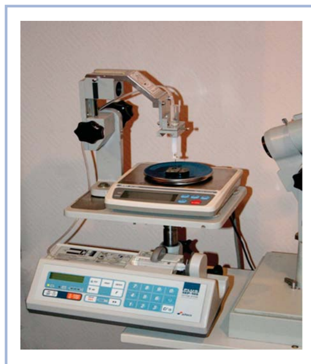
Fig. 1. General view of the stand used for examining viscoplastic properties of biological tissues.
