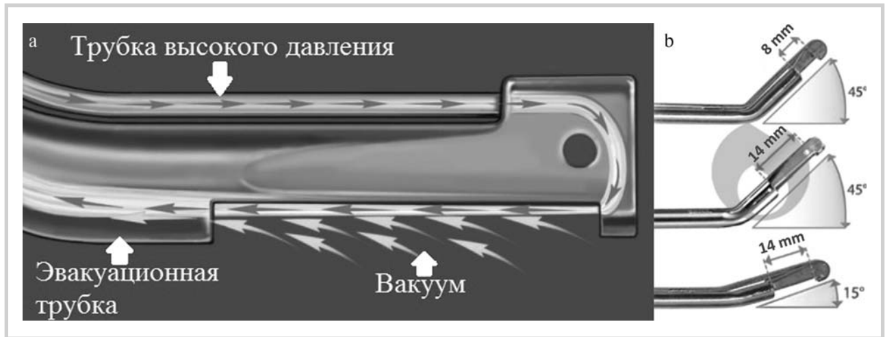
Fig. 2: a — Venturi effect, b — Variants of manipulator handle bending (explanations in the text).
